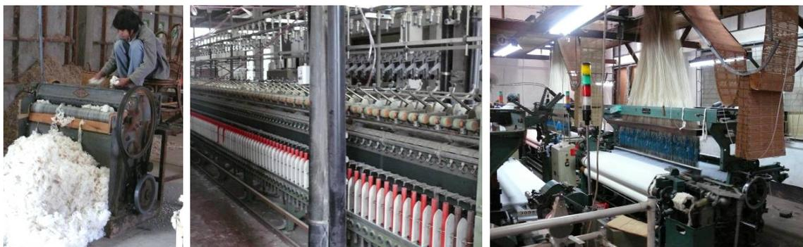
*Photo 5: from left to right: Ginning in Luang Prabang Cotton Enterprise; spinning unit (not functional) and mechanical loom (weaving imported yarn) in Lao Cotton Company.*
